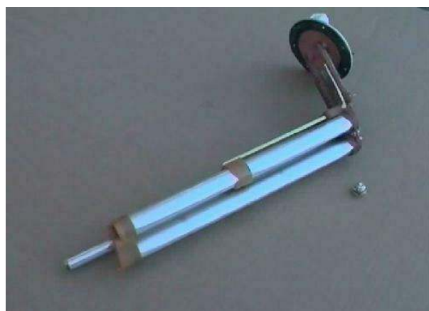
This time the internal alloy tube is removed from the outer alloy tube by sliding out through the bottom.
