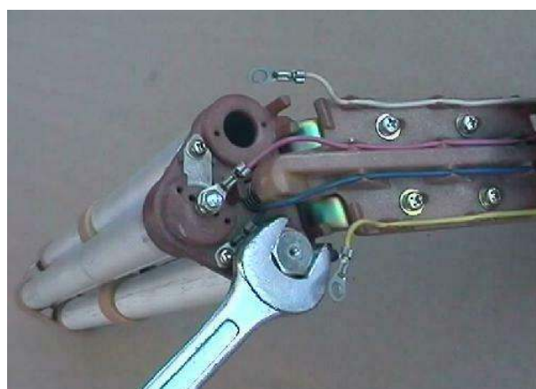
By using a 14 mm spanner, undo the top nut from the other outer alloy tube.
