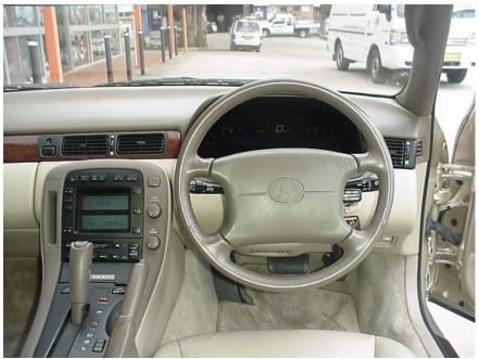
Blank switch between TRC and Height is only distinguishing feature on a '32 without looking at mechanicals. Outside the car look for the rear steering rack above the diff, in the engine bay look for rubber shock boots that say Active and UZZ32 prefix on firewall chassis number.
