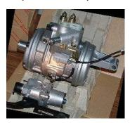
new compressor at the back, EPR valve at the front. The Soarer aircond compressor doesn't turn off and on during operation - it turns the whole time, the EPR valve changes the load on the compressor - when it's cold enough inside the EPR doesn't circulate the gas anymore - reducing load on compressor.
